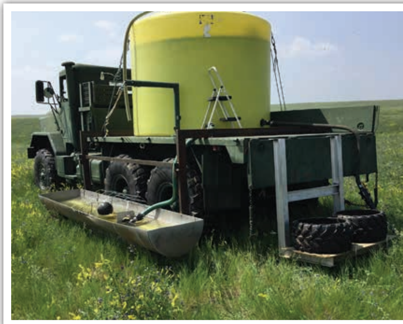
Jeff Brown made a portable water rig using an old Army 6x6 truck. The tank holds 4,000 gallons and can be driven anywhere on the ranch to supply water in far pastures.
