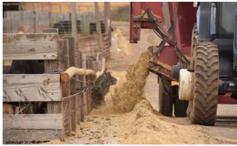
Above: This vertical mixer is used in a feedlot to blend long-stemmed hay, corn silage, potato slurry and ground wheat.
