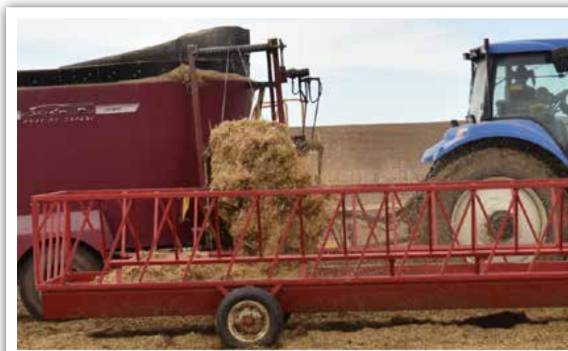
The modifications on this mixer allow the operator to raise the conveyor to the customized height, elevating the feed over the rail of the portable feeder.
