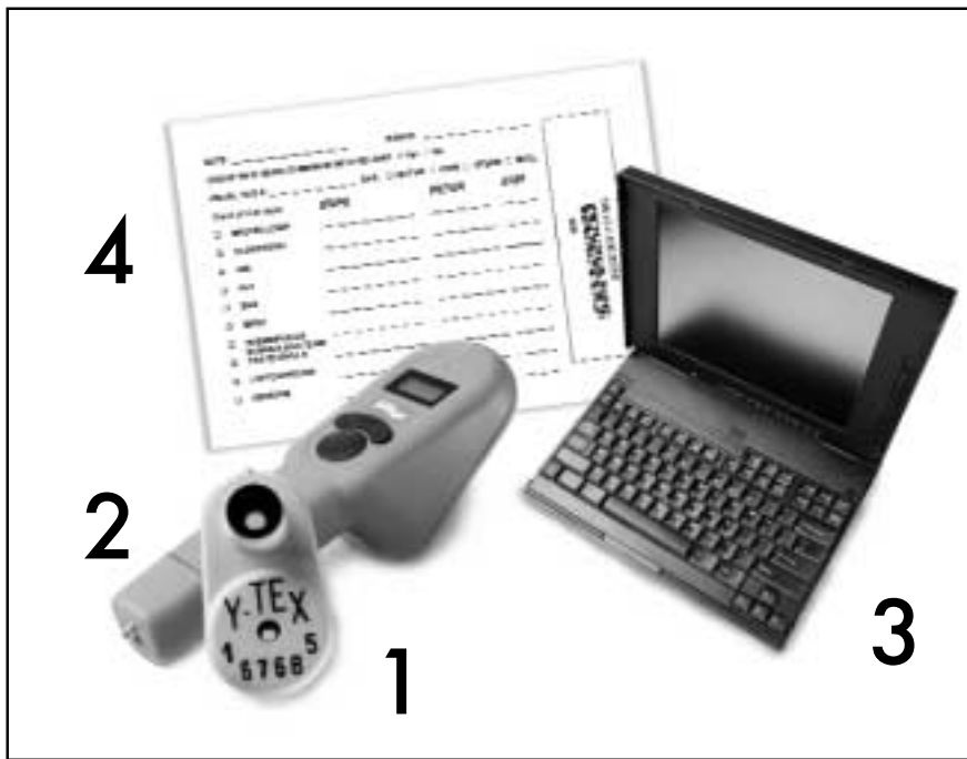
Producers involved in the Iowa Quality Beef program place an electronic-identification tag (1) in the ear of an enrolled animal. Each time that animal hits the chute, the tag is scanned with a hand-held device (2), which calls up the individual's record via computer (3). If a producer doesn't have access to a reader and computer, processing information can be recorded on a bar-coded postcard (4) corresponding to the ear tag. The postcard is sent to the ICA office in Ames, where staff scan the information into the database. (Items are not shown to scale.)
