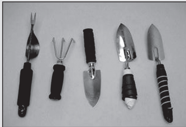
Tools with added padding can be easier to grasp, especially if hand strength is limited.
