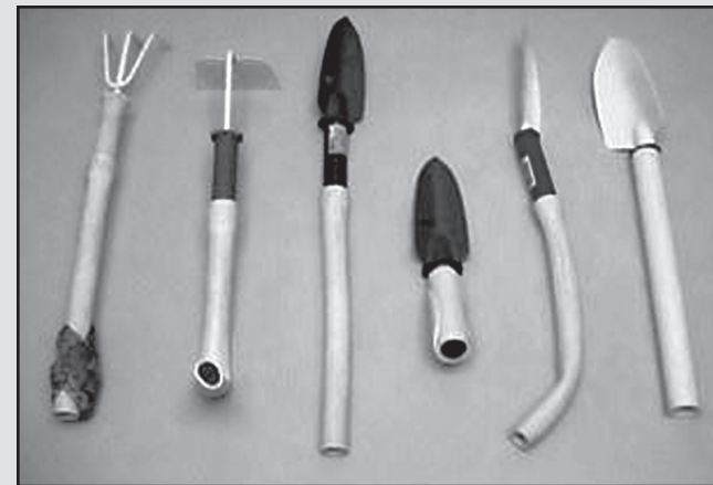
Extending a tool's handle can improve leverage, making it easier to use.
