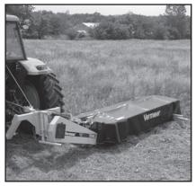
The cutting discs on the cutter bar are all self-contained and prepacked with their own set of gears, bearings and lubricant for longer operating life, according to the release. An exclusive Quick-Clip® Blade Retention System significantly reduces the number of replacement parts required and allows operators to change or reverse an entire set of blades in minutes. All 40 Series
