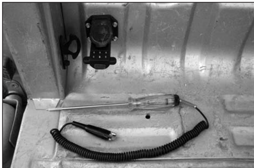
A trailer emulator and test light are handy and valuable tools for isolating electrical problems.
