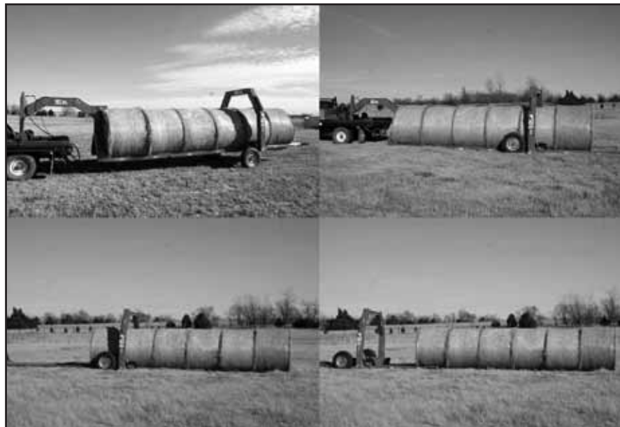
Available with either a gooseneck or a bumper pull, the 2EZ trailer can collect up to six bales of hay, one at a time from wherever they sit, haul them miles over fields or roads, and then gently set them down — all at once in a stack, or one at a time, for feeding.
