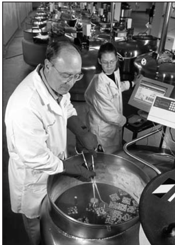
National Animal Germplasm Program coordinator Harvey Blackburn and technician Ginny Schmit place germplasm samples into a liquid nitrogen tank for long-term storage.
