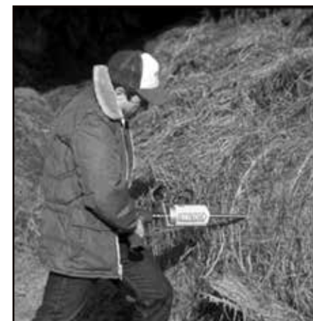
A forage probe is essential for collecting a representative sample. For large round and square bales, the probe should penetrate at least 18 inches (in.) into the bale and have an internal diameter of at least \frac{3}{8} -in.
